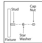
Tuck electrical wires into electrical box and position fixture over studs on mounting bracket assembly. Secure fixture in place with star washer(s) and cap nut(s).
